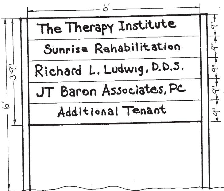
1660 HASLETT ROAD EXISTING SINGLE FACE NON ILLUMINATED WALL SIGN TO BE RELOCATED AS DOUBLE FACE GROUND SIGN. 22,5 D
