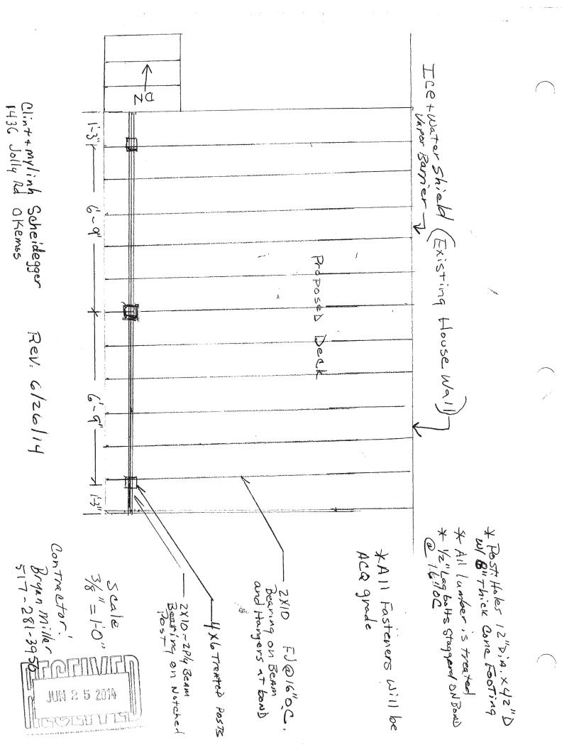
38'' Railing Detail 2x2 Balusters @ 4"O.C. 244 Car 9×2-D 2 0 2-Ply Beam Notches + Bolted To Post Bryan Miller 1436 Jally Rd. JUN 2 5 2014
