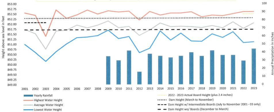
Lake Measurements are in feet and hundredths of feet. 0.01 feet = 0.12 inches or about an eighth inch. 0.10 feet = 1.2 inches. 852.29' - 851.72' = .57' = 6.84 inches (Height of the boards in the dam from March to November 14).
