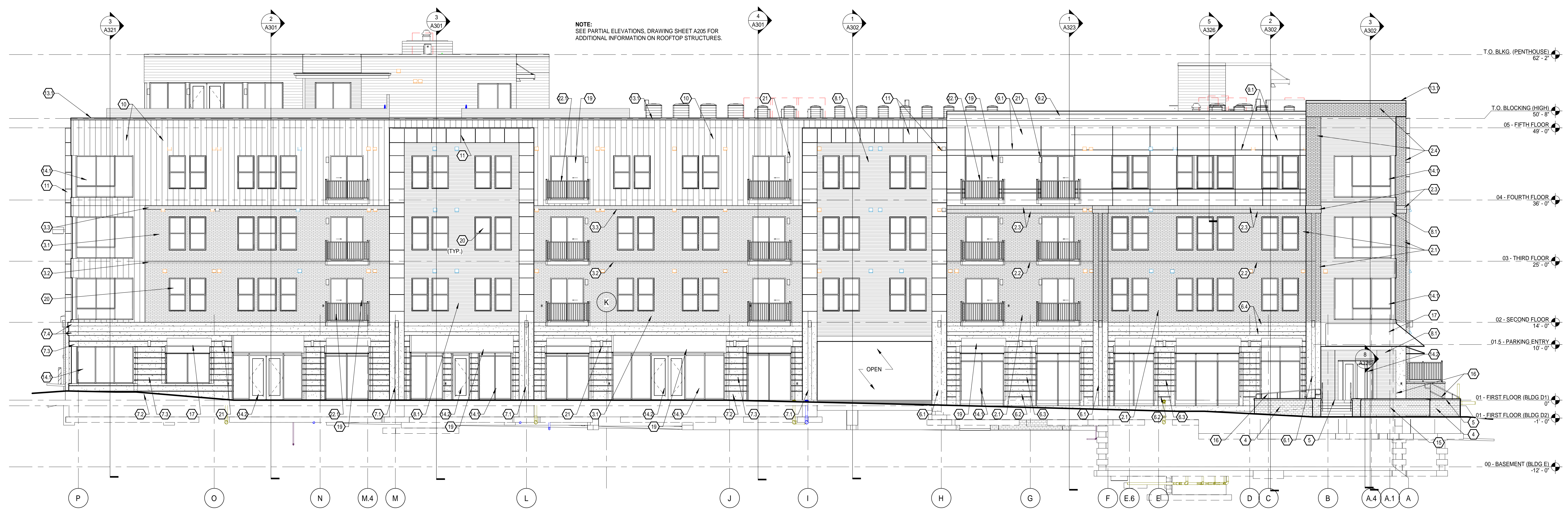
1 SOUTH (HAMILTON ROAD) ELEVATION - BUILDING 'D' SCALE: 1/8" = 1'-0"
