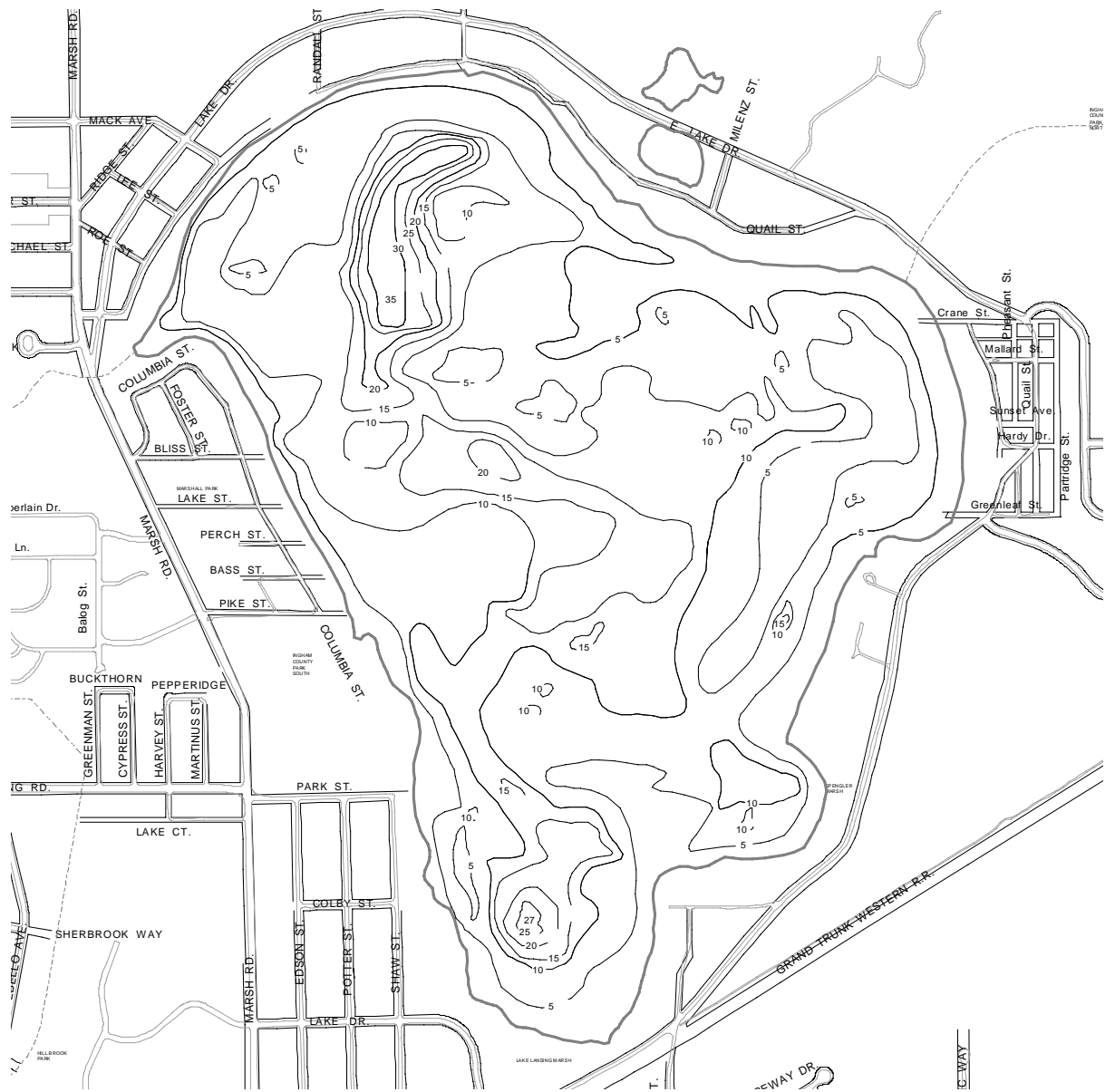
Figure 2. Lake Lansing depth contour map. Depth contour map prepared by Michigan Department of Natural Resources (DNR) based on survey and soundings conducted by Engineering and Land Resource Programs Divisions of the DNR from April 24 to May 10, 1984.
