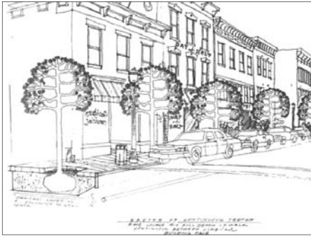
506.B.2 Intent Illustration: The continuous tree trench supports tree longevity and storm-water management.
