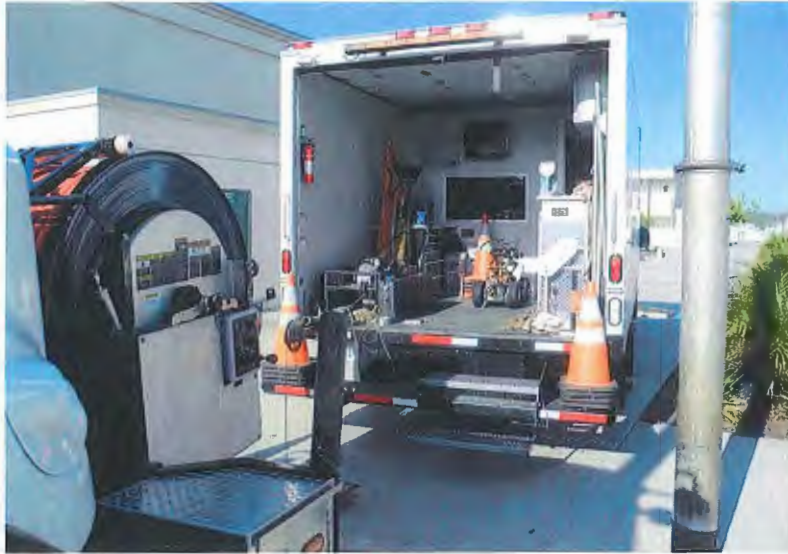
Sewer Camera Truck
